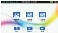
• Can print variable text, QR code and barcode, realizing one object with one code (variable marking). This function only configures individual models.
